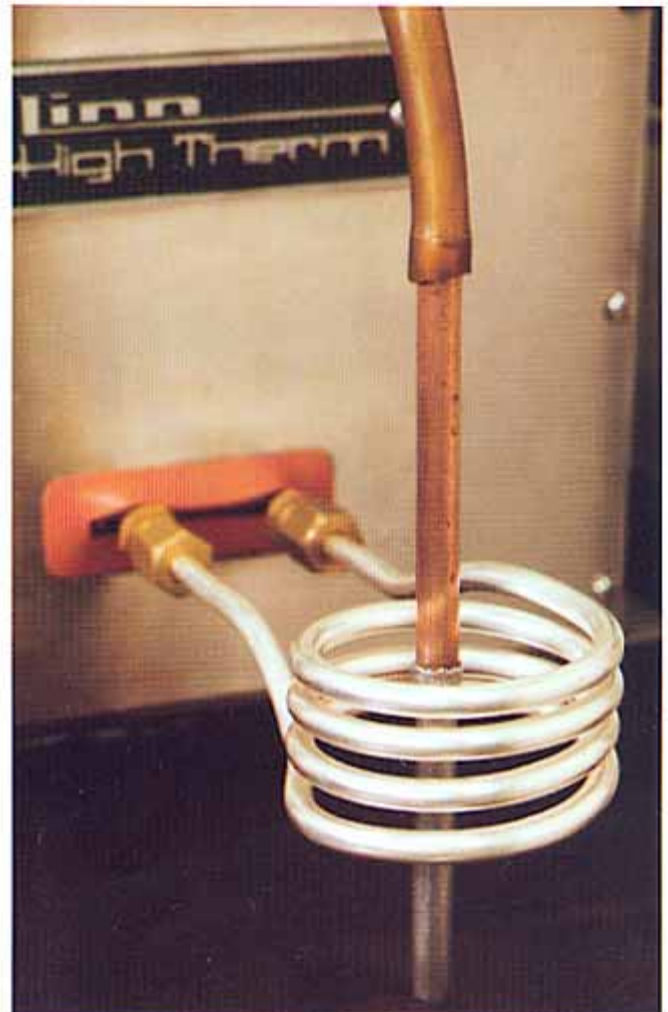
Pict. 13, Diffusion soldering of copper-aluminum joint made with gas shield.
