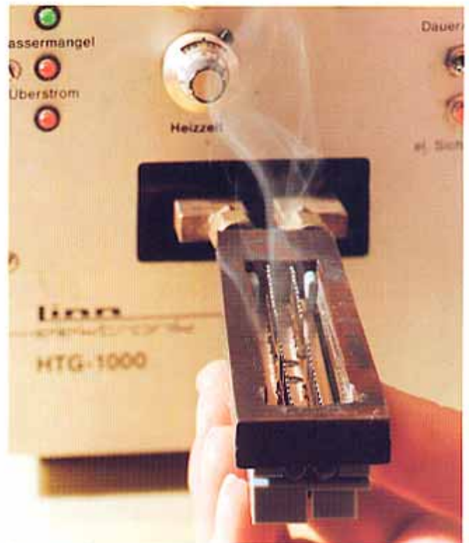
Pict. 19, Simultaneous soldering of 24 connections, in the manufacturing of electrical connectors.
