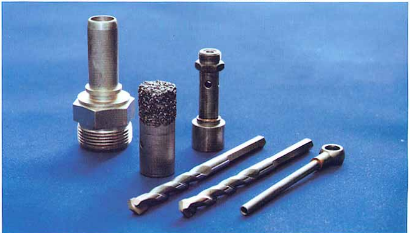
Pict. 17, Gas shielded induction soldered parts. Pipe nozzle – coated semy finished parts – burner jet – drills with carbide inserts – pipe connector.
