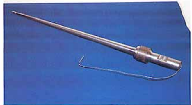
Pict. 16, Measuring probe (1.5 m lg.) 58.5 inches, RF/HF induction soldered in reducing atmosphere using a special heat resistant solder.
