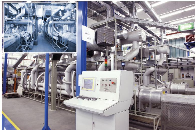
**Fig. 4** Continuous microwave belt dry (50 kW / 20 m)
