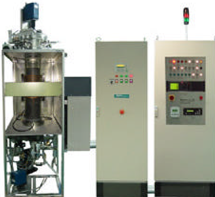
Figure 8: Production crystal growth system for 2" SiC-crystals (4H/6H)
