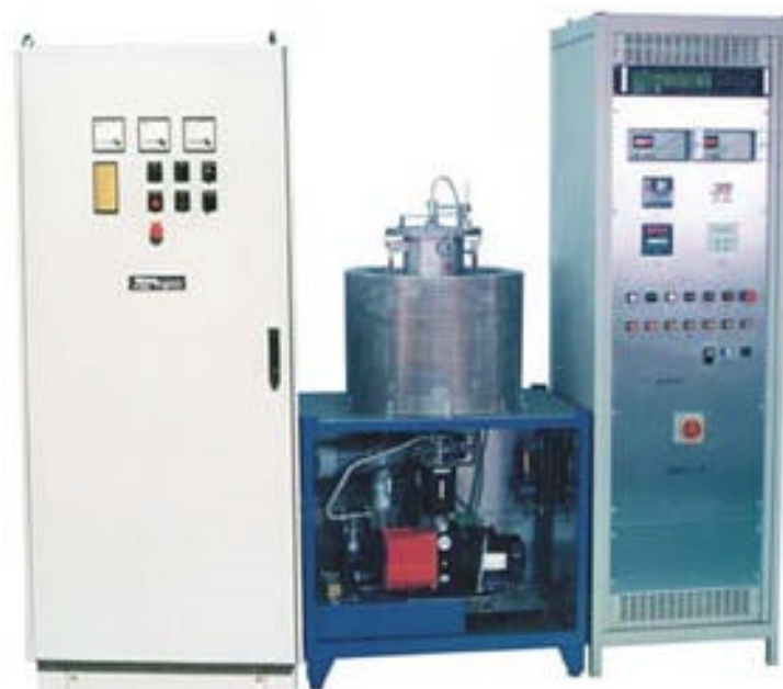
Figure 7: Laboratory- crystal growth furnace for SiC
