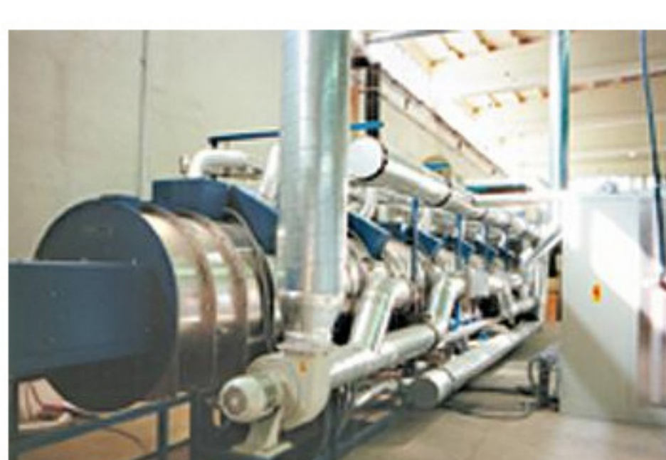
Continous microwave belt furnace e. g. for building material industry 15 m / 60 kW
