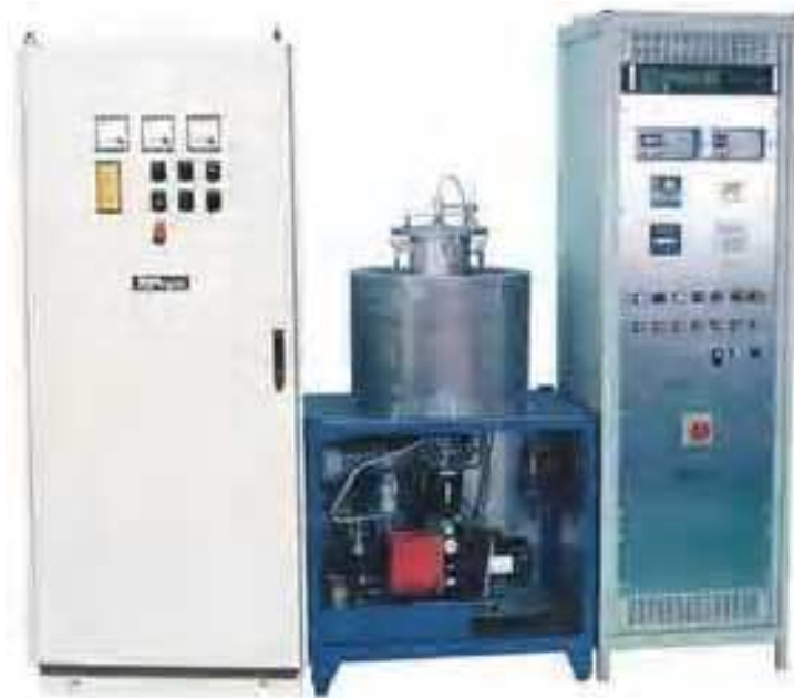
Figure 7: Laboratory- crystal growth furnace for SiC
