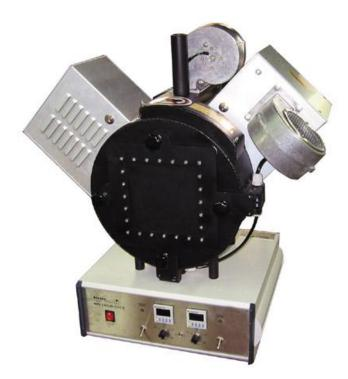
Picture 8: microwave dual frequency furnace, 800 W/2.45 GHz and 600 W/5.8 GHz
