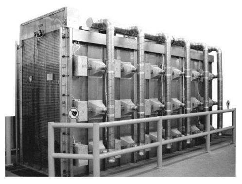
Picture 2: microwave chamber drier, chamber size 21 m<sup>3</sup>, 30 kW
