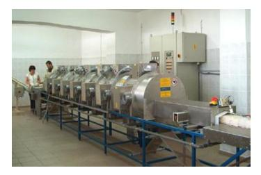
Picture 3: Microwave continuous belt furnace for rice MDBT 21 (Linn High Therm GmbH)
