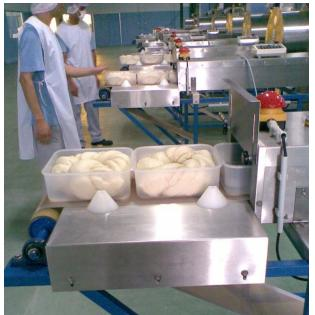
Pic. 2: Continuous Microwave Baking Ovens (Linn Close-up of microwave baked crust-less High Therm GmbH Model MDBT 12)
