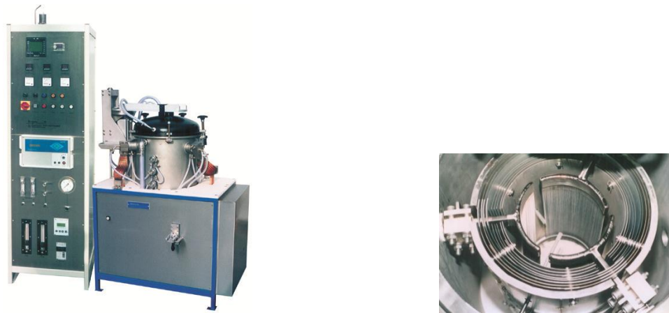
Picture 7 Cold wall furnace KKV 140/270/2000 up to 2200 °C.
