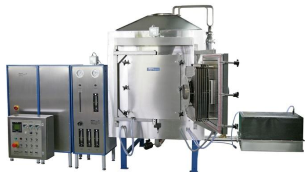
Picture 3 Fibre insulated gastight furnace KF-240 S up to 1200 °C for reduction and sintering of precious metall pellets under hydrogen. Gas recooling by gas/water-heat exchanger for fast cooling. Furnace prepared for clean room installation.
