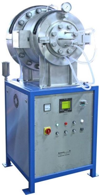
Picture 6: High pressure furnace up to 1000 °C. Operation under pure oxygen up to 100 bar. Heated with molybdenum-disilicide. For development of High-Temperature Superconductiv materials (HTSC).
