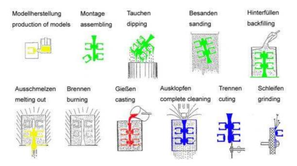
The original model, for example made of metal, will be moulded in silicone or rubber. This original mould reproducible by filling with wax or plastic. Then the parts will be mounted in treeform and the wax model is backfilled with ceramic mass in a moulding ring made of heat-resisting steel. Depending on the material tube slurry the mould will be preheated and fit into the casting machine to fill in the metal.
