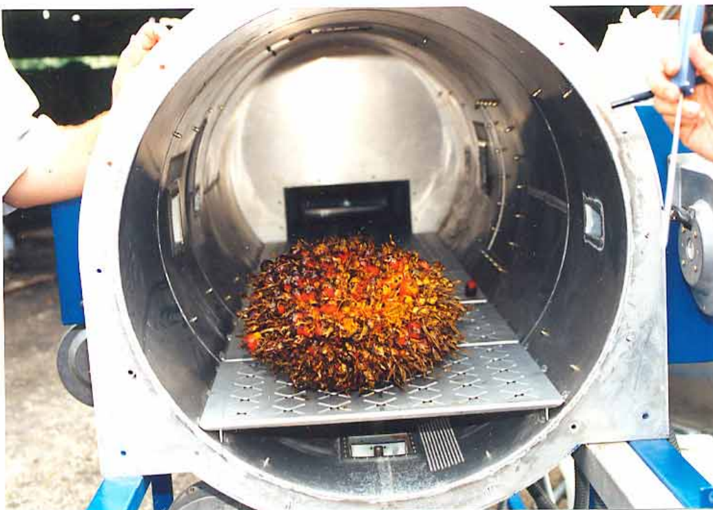
Fig. 2: The Front Cover of Furnace Removed to Accommodate a Whole Fresh Fruit Bunch.
