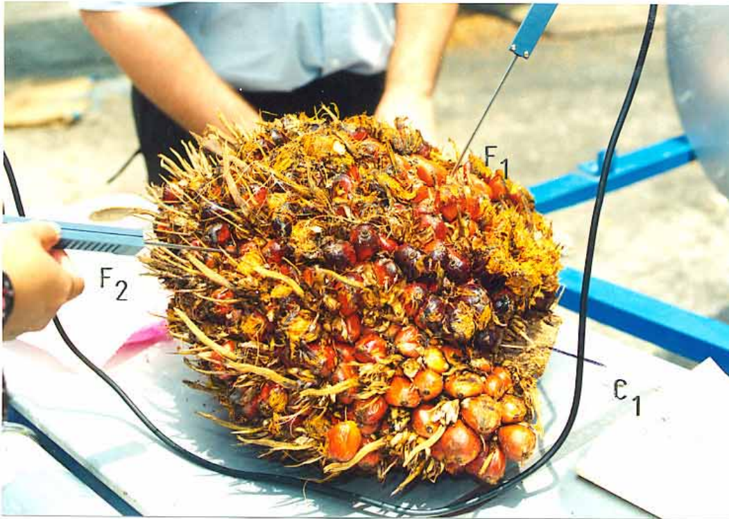
Fig. 3a: Thermocouples Inserted into the Respective Position of the Whole Bunch. F 1 :Outer layer of fruits, F 2 :Inner Layer of Fruits, C 1 :Core of Bunch
