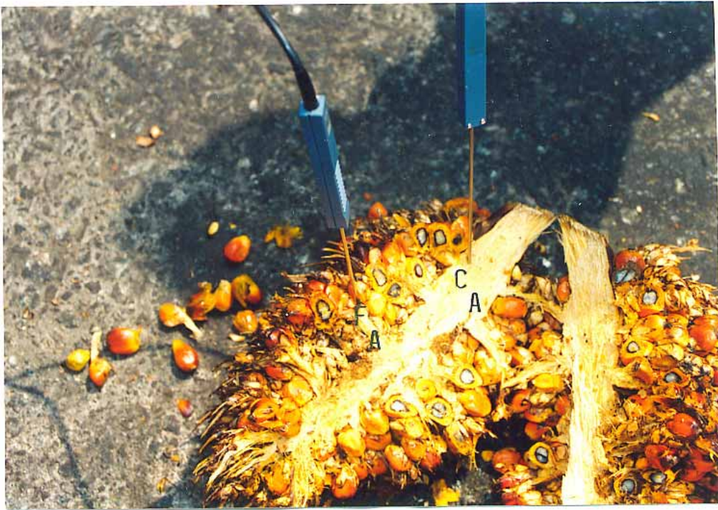
Fig. 5: Longitudinally Axed Bunch indicating the Positions where the Temperatures were taken. C_A : Core, F_A : Innermost Fruits
